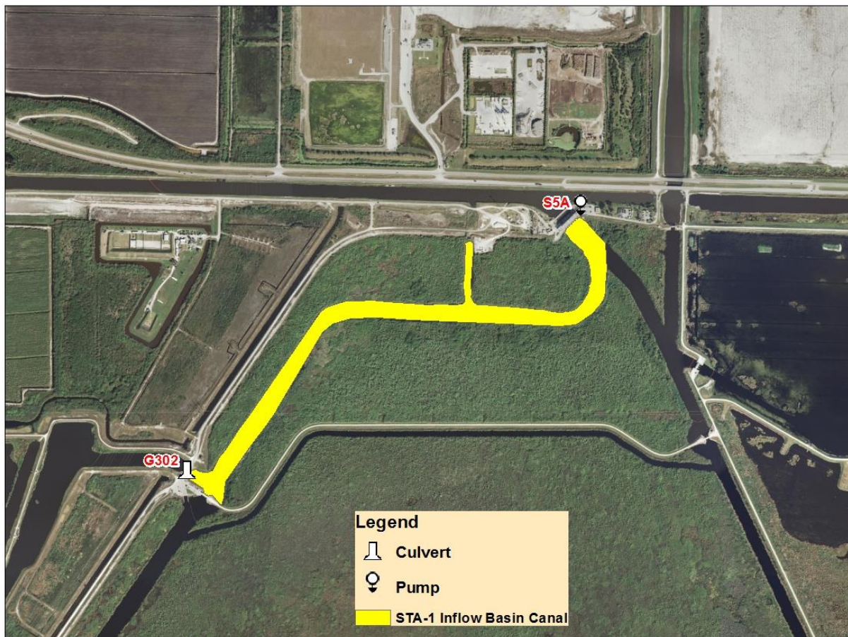
Figure 1-1. Map of the STA-1 Inflow Basin Canal between S-5A and G-302 showing other water control structures.
